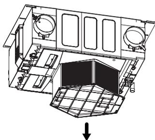
**Step 3** Supporting with your hand, gently remove the heat exchanger, taking care not to tilt it to an angle as water will be present. Clean each face of the heat exchanger with a vacuum cleaner and wash with warm water, take care not to cause damage to the unit. Gently clean the motor impellers on both sides of the unit by using a brush. Ensure heat exchanger is dry before continuing to Step 4.
