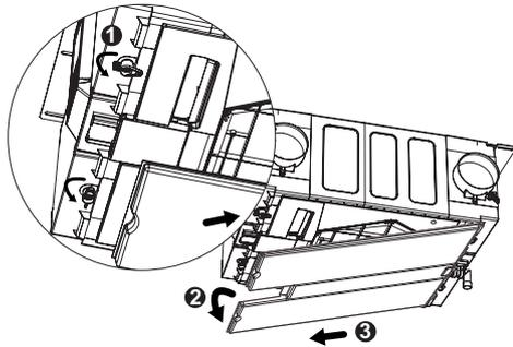
**Step 1** Isolate the unit from the Mains Supply. Rotate and unlock the tabs (1), Slightly pull down the top part (2) of the front panel and pull out (3) of locating tabs and condensate connection located at the bottom of the unit.
