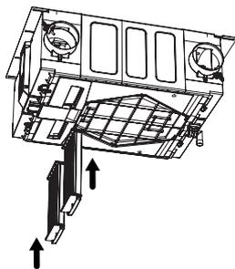
**Step 3** Re-insert new filters into the unit.
