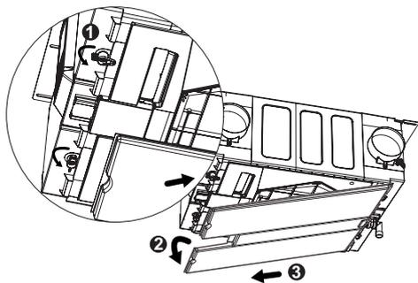
**Step 1** Isolate the unit from the Mains Supply. Rotate and unlock the tabs (❶), Slightly pull down the top part (❷) of the front panel and pull out (❸) of locating tabs and condensate connection located at the bottom of the unit.
