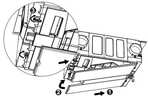
**Step 4** Re-connect the front panel (1) into the condensation connection point and the bottom locating tabs and position back against the unit (2). Rotate the two retaining latches to secure (3). Turn the mains supply back on, Reset Filter Status (See Section 4.1.5). Note details on the Service & Maintenance Log on page 13.
