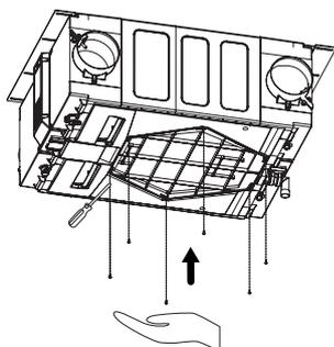
**Step 5** Reposition the panel against the unit and secure with the six locating screws.
