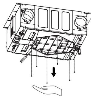
**Step 2** Unscrew the six heat exchanger locating screws and remove panel.
