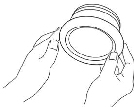
**Step 1** Keep hold of the valve on its outer edge and pull it completely out of the wall or ceiling with a rotating movement. If a rubber ring is fitted: Take care when removing the valve to leave the rubber ring in place.
