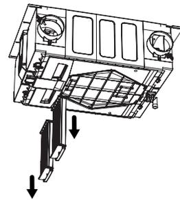
**Step 2** Remove both filters from the unit by the handles.
