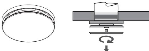
Turn the design cover a quarter **counterclockwise** and then remove it from the valve.
