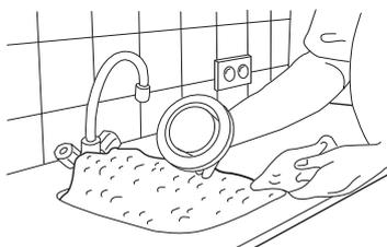
**Step 3** Remove the filter behind the valve (if present).
