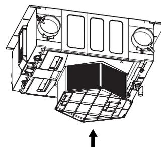
**Step 4** Re-insert the cleaned or a new heat exchanger, taking care not to cause damage. Support in place with hand until completing Step 5.
