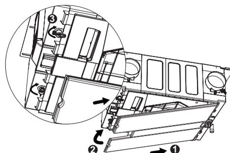
**Step 6** Re-connect the front panel (❶) into the condensation connection point and the bottom locating tabs and position back against the unit (❷). Rotate the two retaining latches to secure (❸). Turn the mains supply back on. Reset Filter Status (See Section 4.1.6). Note details on the Service & Maintenance Log on page 13.
